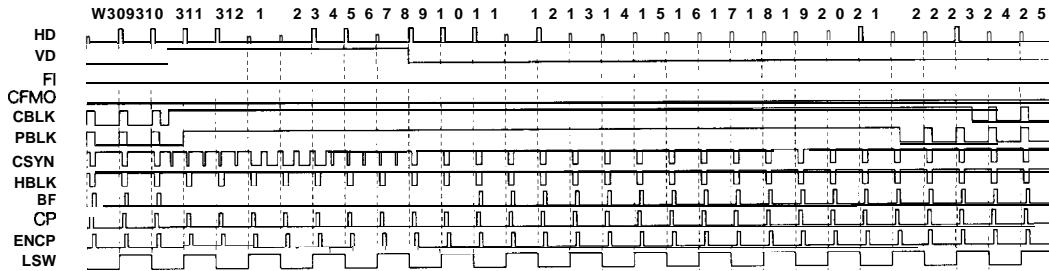
**VERTICAL PULSE FOR DRIVING CCD < NTSC >**
