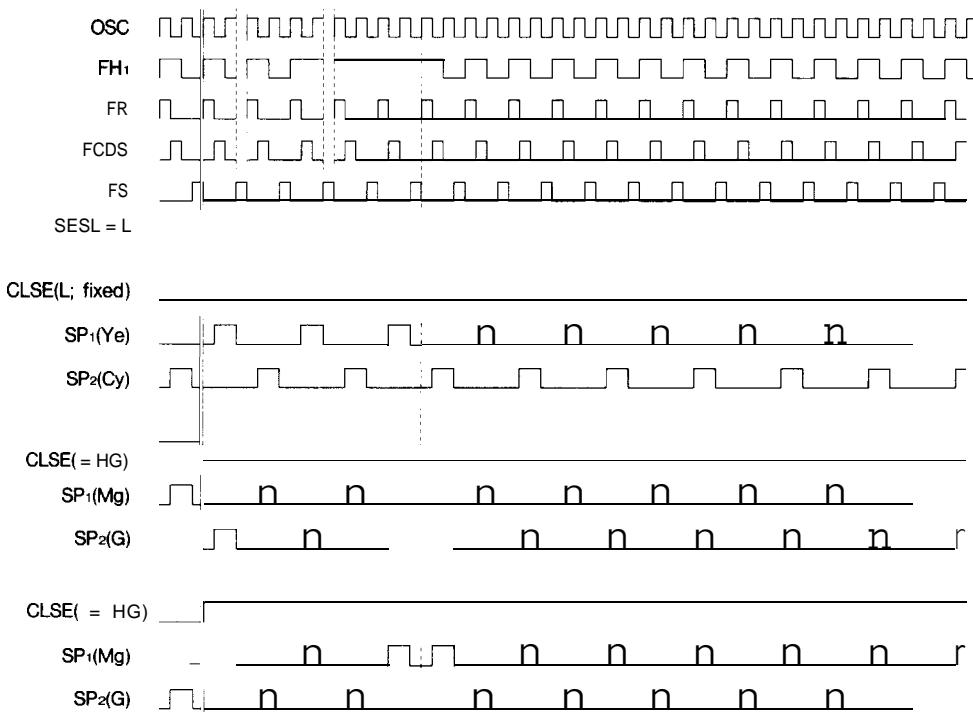
The SP<sub>2</sub> pulse is delayed about 35 ns at SESL= H
