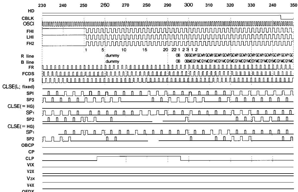
At  $\text{SESL}=\text{L}$  : When  $\text{SESL}=\text{H}$ ,  $\text{SP}_1$  and  $\text{SP}_2$  is delayed about 35 ns.
